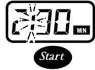
**NOTE:** For some models, when the power head is lifted during cooking, the unit may automatically go to PAUSE mode. Fan and heater will stop working, but the remaining cook time and power setting are still in the memory. Once the power head is put back on, you need to push **START** to resume cooking.
